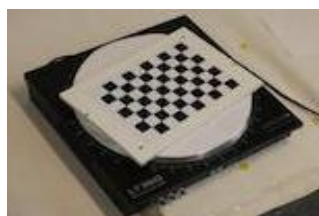
Figure 3. A standard chequerboard calibration target
